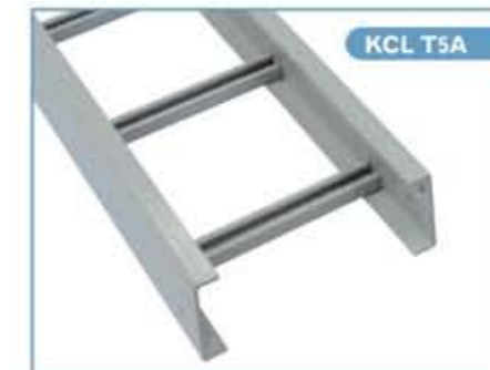
KCL T5A C-Type Channel (150 x 40 x 6 mm) Range: 150 - 1200mm Wide Rung: 40 x 20 x 3.8 mm with Fasteners
