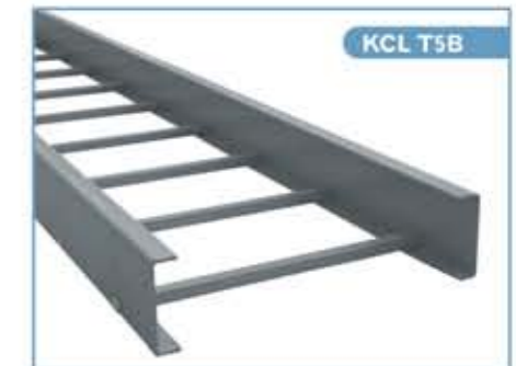
KCL T5B C-Type Channel (150 x 40 x 6 mm) Range: 150 - 1200mm Wide Sq.Pipe: 25 x 25 x 3 mm Nylon Bush
